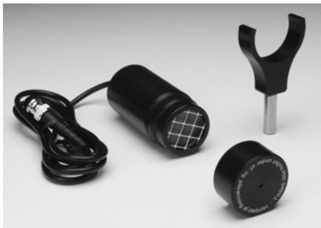
This GM tube is suitable for measuring low levels of radiation where the small number of counts would give rise to large uncertainties. The GM tube has quite a large window, and will typically give 3 times higher count rates than a standard GM tube – for instance in half-life measurements with the isotope generator (no. 5112.00). This tube is also very well suited for detecting radon daughters.
