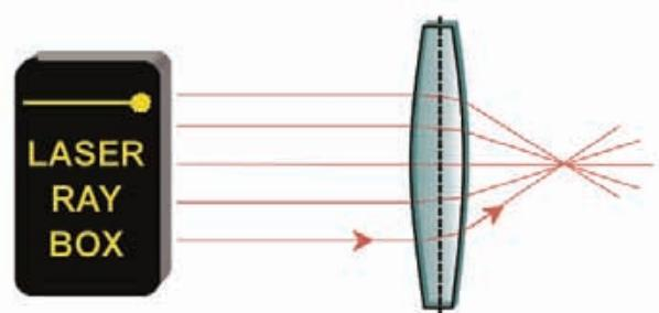
**E17b Light beam passing through glass convex lens
