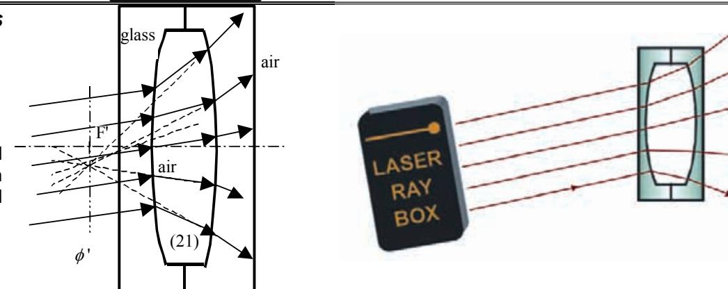
**E20a Light beam passing through air concave lens – the rays are parallel to the optical axis**
