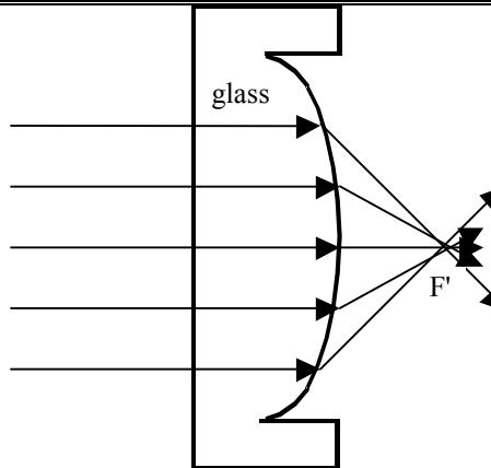
The beam is convergent after passing the boundary. Parallel rays meet in one point of the optical axis – **figure focus** F'.
