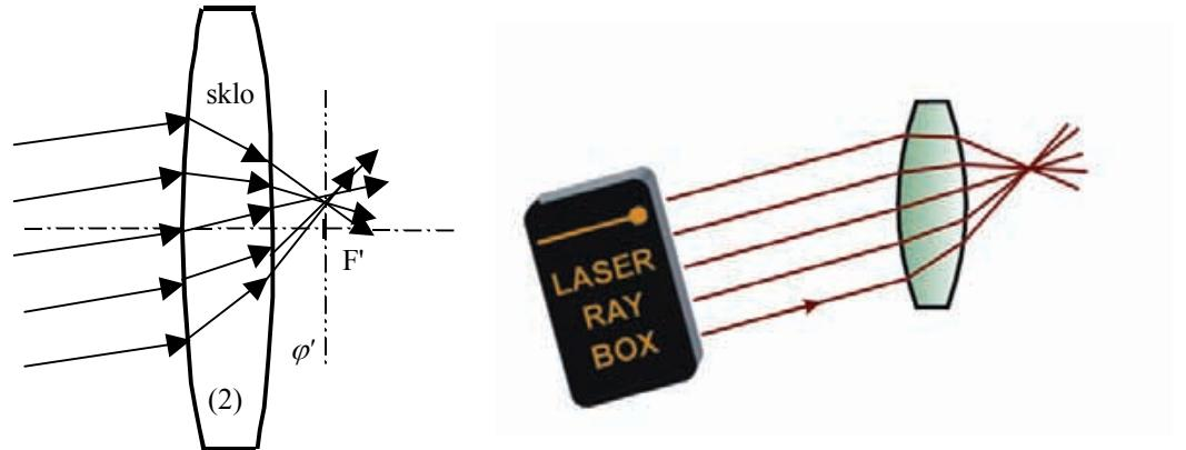
**E17c Light beam passing through thick glass
