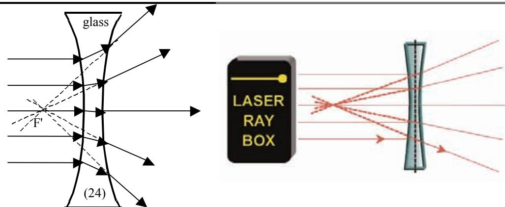
**E18b Light beam passing through glass concave lens – the rays are non-parallel to the optical axis**
