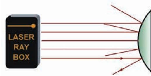
**E4b** *Reflection of light rays on convex mirror – rays are non-parallel to optical axis*
