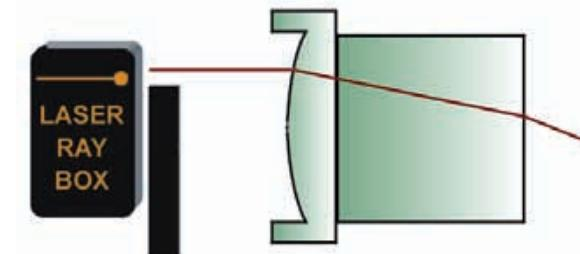
**E13b Light beam passing through concave air – convex glass boundary**
