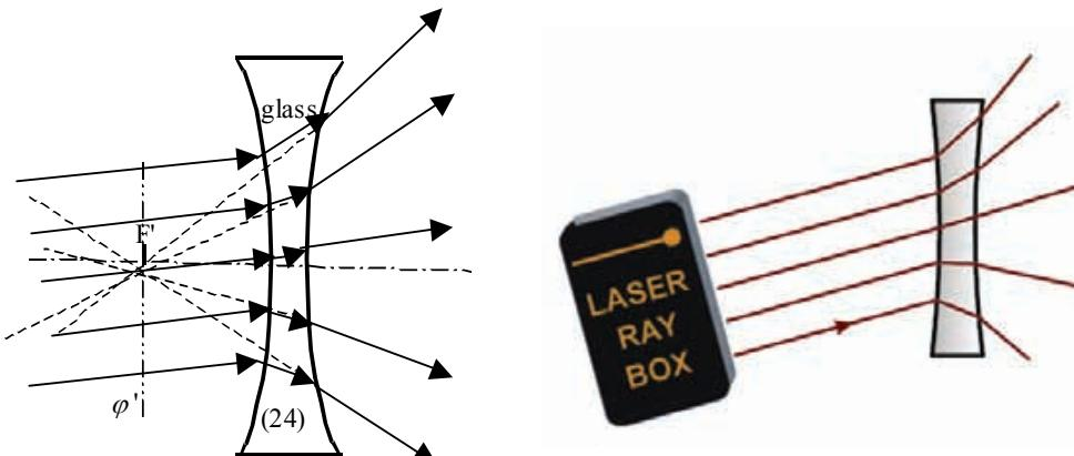
**E19a Light beam passing through air convex lens – the rays are parallel to the optical axis**
