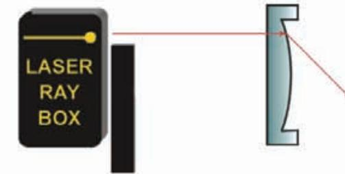
**E16b Light beam passing through convex glass – concave air boundary**
