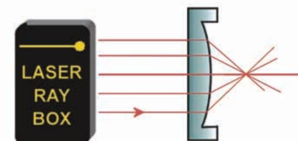
**E17a Light beam passing through glass convex lens – beam is parallel to the optical axis**
