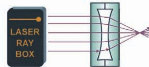
**E20b Light beam passing through air concave lens – the rays are non-parallel to the optical axis**
