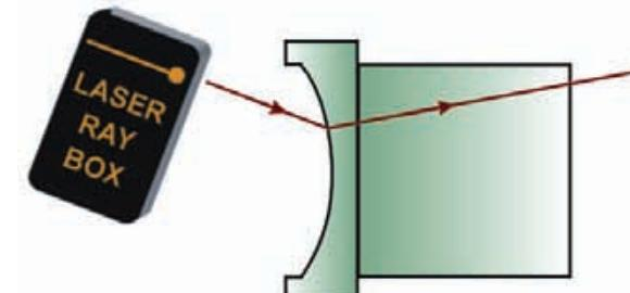
**E14b Light beam passing through convex air – concave glass boundary**
