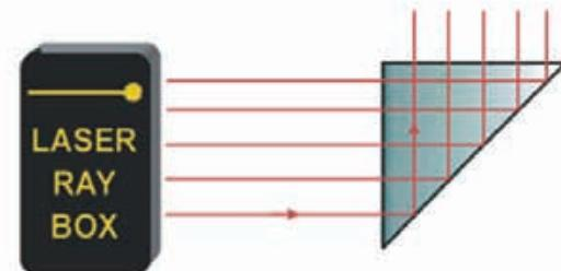
**E11b** *Reflection of light on two edges of glass prism*
