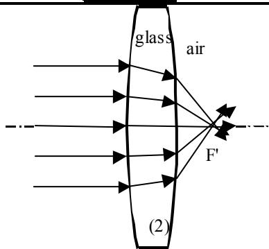
A convex glass lens behaves as a **convergent optical system** and the rays meet at figure focus F' after passing through the lens.
