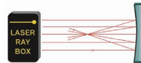
**E3b** *Reflection of light rays on concave mirror – rays are non-parallel to optical axis*
