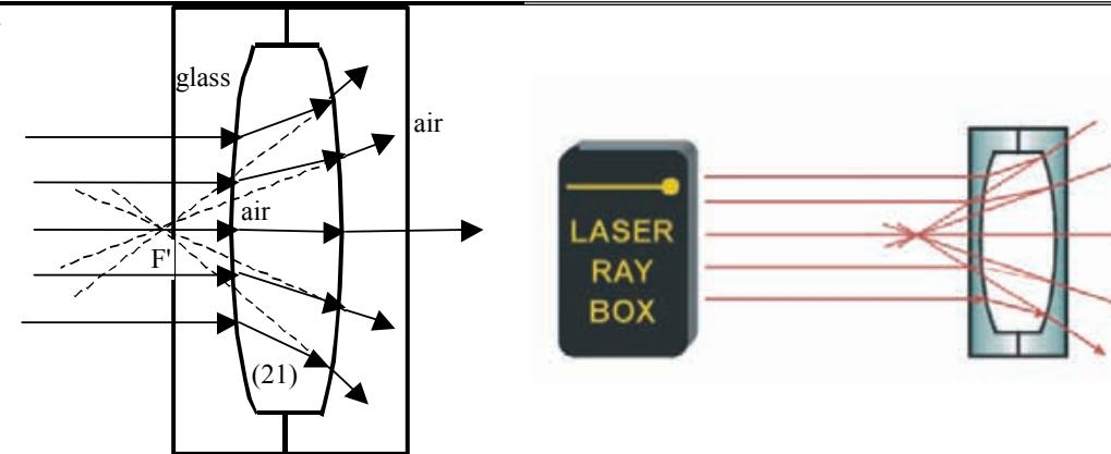
**E19b Light beam passing through air convex lens – the rays are non-parallel to the optical axis**
