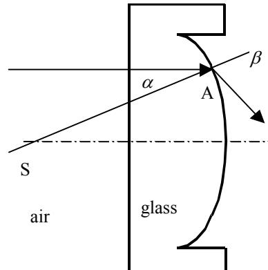
When a ray impinges the boundary at point A, refraction away from the normal is observed. The normal is defined as the line from point A to the centre of boundary curvature S.
