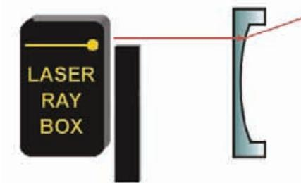
**E15b Light beam passing through the concave glass – convex air boundary**
