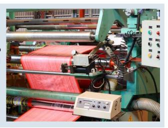
Photograph shows sensors on a textile machine.
