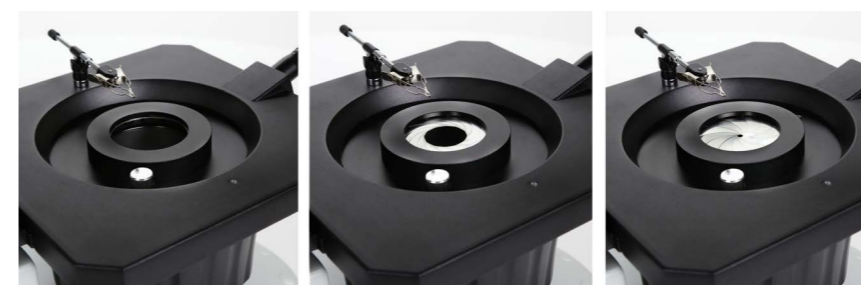
the adjustable iris enables easy light and contrast control
