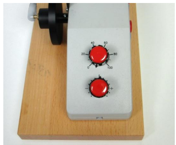
Figure 5: Control knobs for adjusting the excitation frequency. Upper knob: "coarse"; lower knob: "fine".
