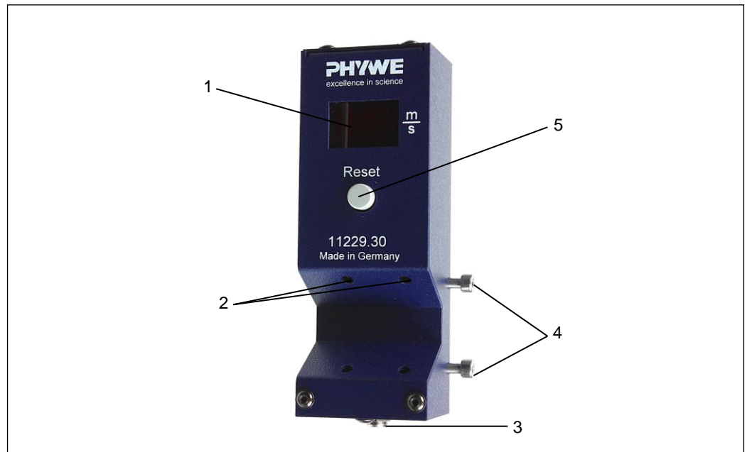
Fig. 1: Speed measuring attachment 11229-30.
