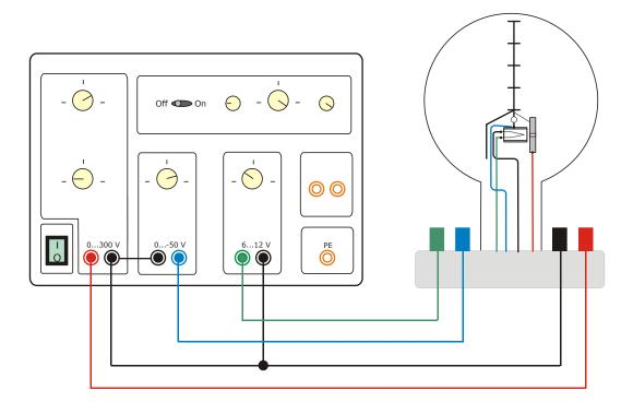
Fig. 1 Electrical connections from the fine beam tube to the DC power supply unit 300  $\rm V$
