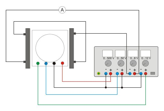
Fig. 4 Electrical connections from the fine beam tube to the DC power supply 500  $\rm V$
