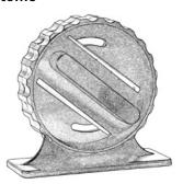
The microtome is a very safe and easy to handle instrument to sectioning biological material. With the knife a suitable piece of botanical material or dead animal is cut. This piece of material is passed through one of the openings of the microtome. It may be hold by the tweezers. Now the handle is turned to cut of a thin section from the material. The section can be taken by the tweezers and then prepared for further investigations.
