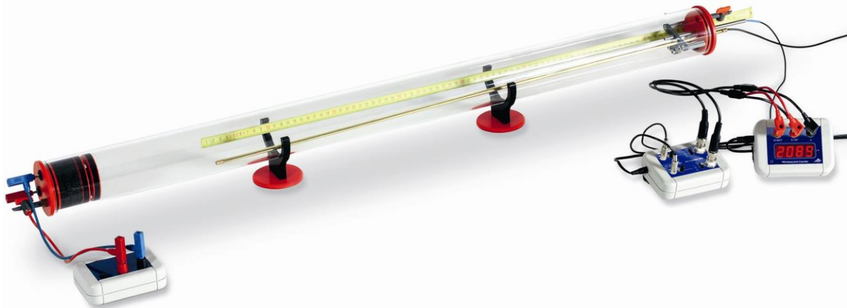
Fig. 1 Determination of speed of sound by measuring the time it takes for a sound pulse to cover a given distance
