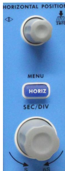
Fig. 11 Horizontal Control Zone
