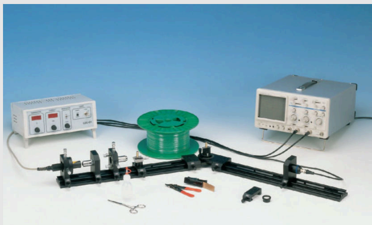
Experimental set-up: Fibre optics with monomode fibre
