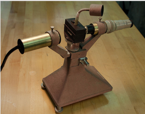
Oil drop experiment apparatus
