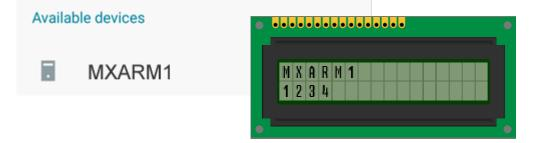
The name of the AllCode Robot Arm appears on the LCD when powering on the Robot Arm to let you know the Bluetooth name of the robot you want to connect to.
