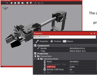
The component comes with a fully operational simulation allowing us to create and test programs before we move to the hardware.
