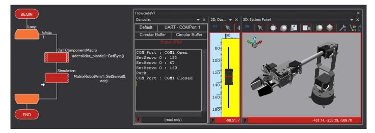
The selected communications (COM) port is automatically opened when you start the simulation. The motors automatically return the arm to the parked position before closing the port when you end the simulation.
