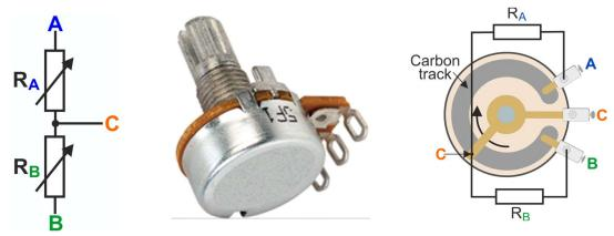
The circuit diagram shows the structure of a typical 'pot' having three terminals, A, B and C.
