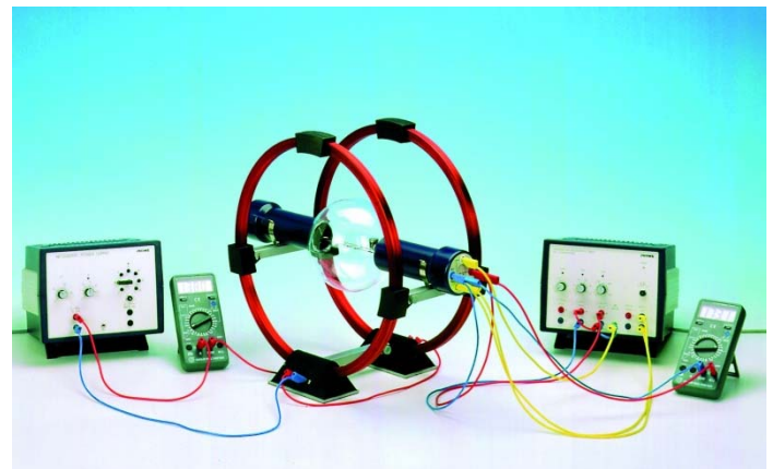
Fig. 3: Experimental setup for determining e/m with the narrow beam tube.
