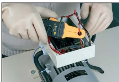
Faults can be looked for inside the student unit and in the motor terminal.
