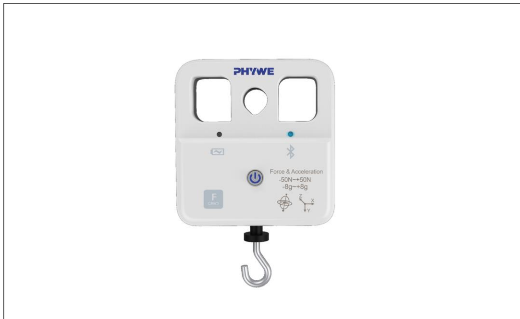
Abb. 1: 12943-00 Cobra SMARTsense Force & Acceleration
