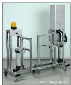
The gates POA-1 and POA-2 are supplied with an autonomous wheeled frame comprising a solar panel 25W-24VDC and two spotlights simulating the sun.
