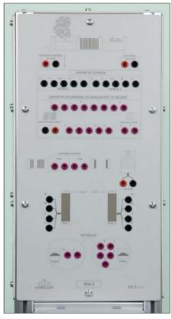
Connection console with printed diagram
