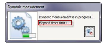
Press the 'Stop' button in the progress window to stop the dynamic measurement.
