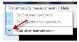
The check marks for dark/reference spectrum indicates, that the corresponding spectrum was already captured
