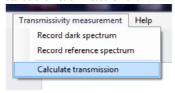
In order to stop the transmission measurement, uncheck the 'Calculate transmission'
