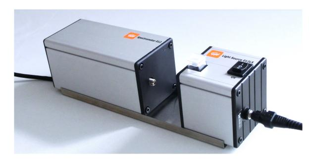
A cuvette containing a sample solution should be inserted into a hole.
