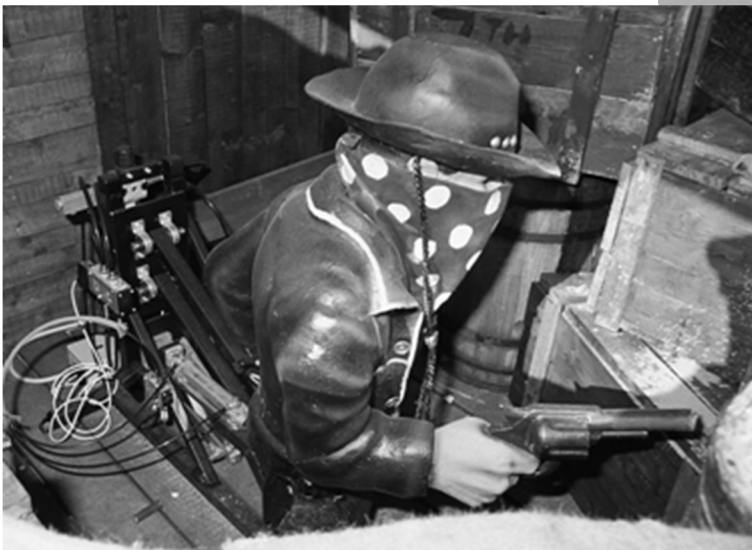
Pneumatically controlled animated bandit figure
