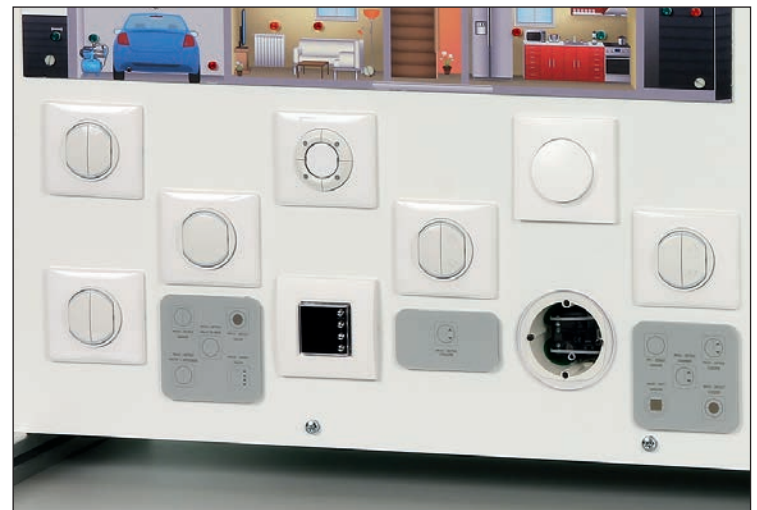
All of the configurable standard and MyHome switches are integrated on the front panel. A translucent plate on the universal adapter covers the connectors and protects against electrical contacts. The programming of MyHome components does not require any disassembly on said components, thus improving their lifespan.
