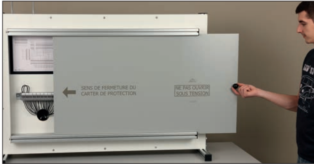
The components are wired on the rear panel via industrial terminals to prevent wear of the component terminals. A housing protects access to industrial terminals during tests with power on. Removable wiring diagram.
